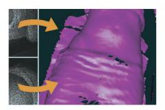
A pseudo-random speckle-pattern is projected onto the patient's skin. The cameras use stereo-vision techniques and a triangulation process to create a high-res 3D surface of the patient that comprises several thousand points (displayed on the monitor).
